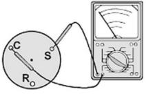
Figure 1: Compressor winding test
